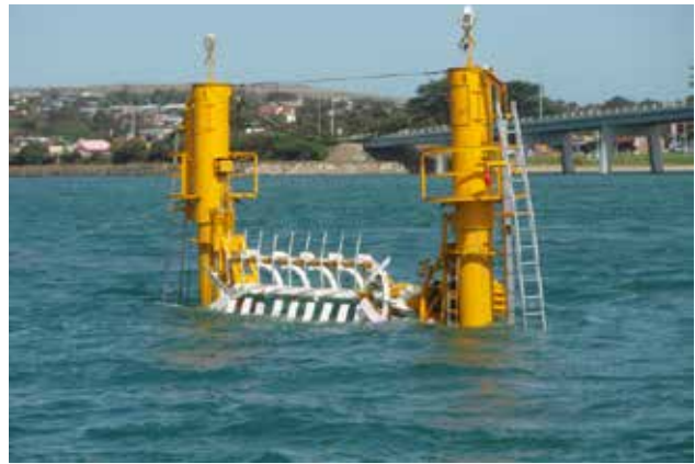
An underwater tidal renewable power generation turbine developed e3k. Photo courtesy: Duncan Gilmore.
