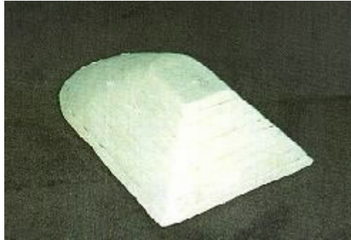
Figure 3.1 A part cut with sloping layer edges.
